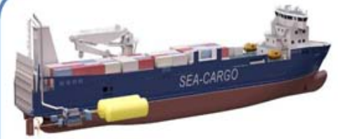
LNG powered vessel design (source: DNV)
