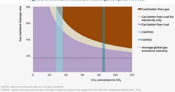
Figure 2: GHG emission intensity of natural gas compared with coal
